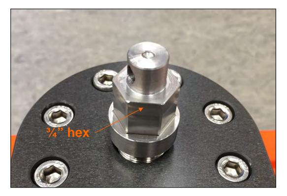
Once the retaining clip and ratchet have been removed the squex can still be operated by using a 3/4" spanner
