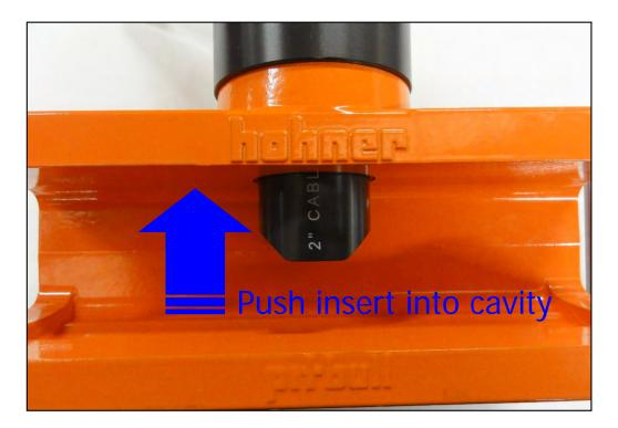
Push the selected insert into the cavity in the centre of the upper wall of the channel The tip of the 'squex' and each insert contain magnets to help hold one to the other Rotate the 'squex' until it mates with the insert; the insert should now be held in place \*NOTE\* PLEASE APPLY FRESH ANTI SEIZE PASTE TO THREAD OF SQUEX WITH EACH NEW DEPLOYMENT
